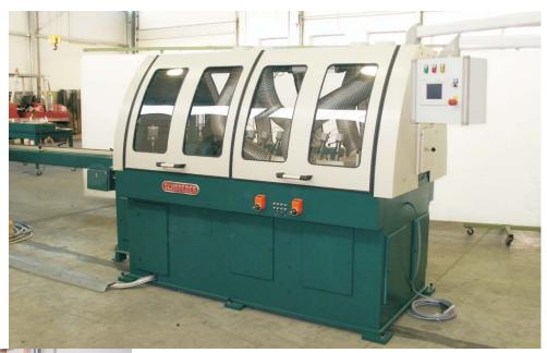
4 roller feeding unit with pneumatic control and automatic feed speed control system.
